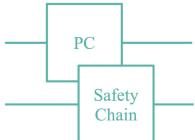
A Safety Chain based on a certified PLC (Programmable Logic Controller) is independent from the main computer. It uses very simple algorithms and can perform emergency stops should the main computer fail to anticipate the potential collision.
